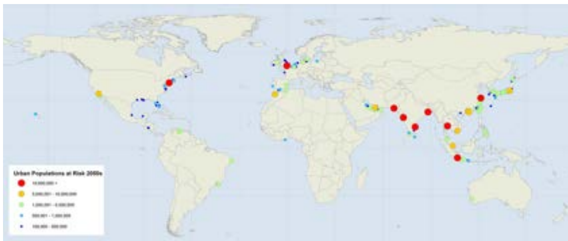
Figure 8. Cities whose nearby power plants are vulnerable to coastal flooding as a result of 0.5 metres of sea level rise in the 2050s.
